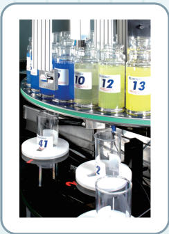
Diluting Stock Solution Making a dilution of solution by reading the RFID tag from the bottle to prevent the human error, reduce time-consuming and tedious, to achieve the goal of high-throughput and reliable.
