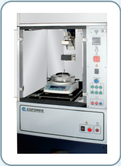
Making Standard Solution Making a standard solution by reading the RFID tag from the dye can and bottle. It can prevent the human error, convenient and reliable.
